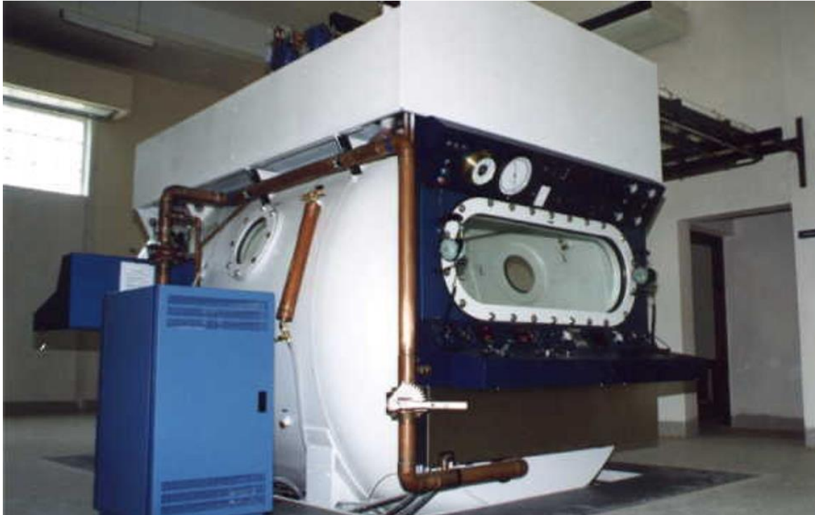
PHS Model ATR-6 (cylindrical), Aviation Training Altitude Chamber, Dual Compartment, installed at Bangladesh Air Force base in Dhaka, Bangladesh
