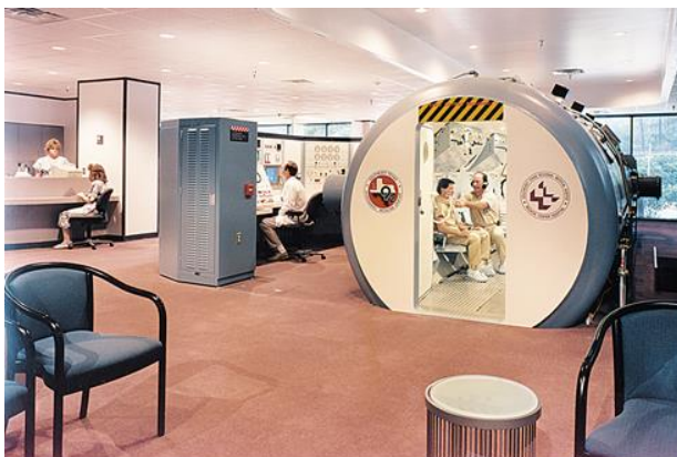
PHS 9600 Series – Dual Lock – Cylindrical – 6 ATA Working Pressure – Rated for 12 patients and upto 3 attendants, installed at Conroe Medical Center, Dallas, TX
